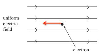
Draw an arrow on the diagram to show the direction of the electrostatic force that acts on the stationary electron.
