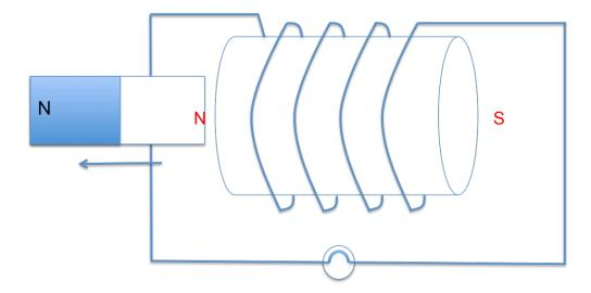
(d) Add labels to the diagram to show the north and south pole of the solenoid as the magnet moves away.
