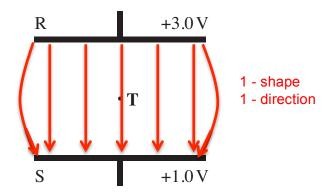
(a) On the diagram, sketch the electric field between R and S, showing its direction. Point T is mid-way between R and S.
